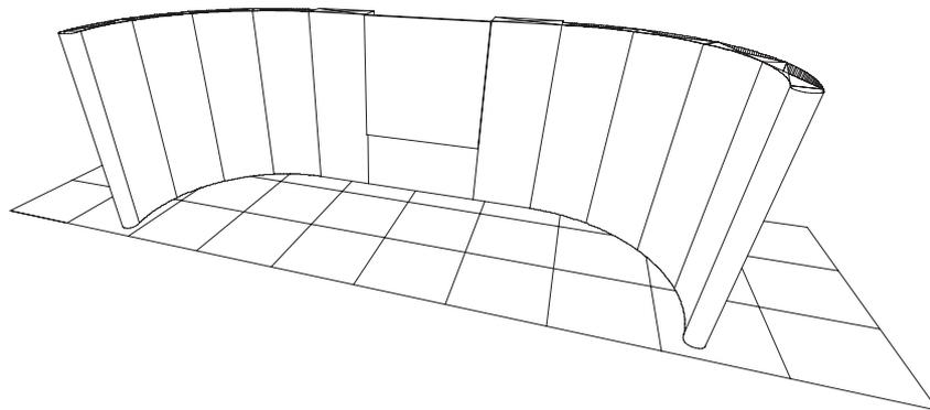
Small (2 X 2) Screen Conference Kit with 4 off 3 X 2 Curved P300 in a 'gullwing' shape on each end. There is also a straight 1 X 4 frame hinged over the screen.
