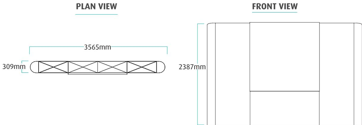
The smaller sized CK is based on a 3 X 4 Premier P300 flat frame. This accommodates a 2 X 2 quad projection screen.
