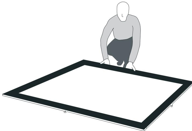
The screen support frame is supplied with magnetic tape on the rear. The screen is applied up to the magnetic bars on the Premier P300 U-shaped frame.
