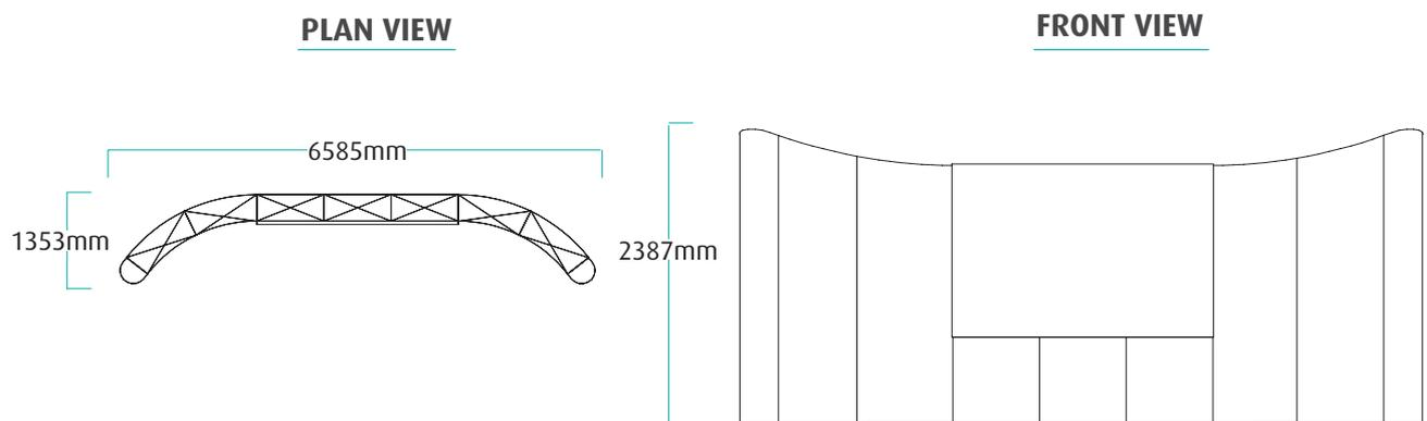
The larger CK is based on a 3 X 7 Premier P300 curved / flat frame. This accommodates a 2 X 3 quad projection screen. The projection screen is available for front or rear projection.
