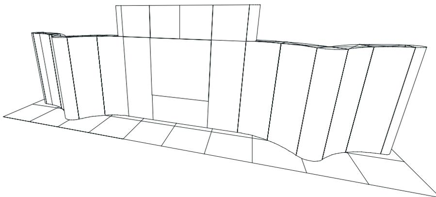
Small (2 X 2) Screen in a Premier P300 4 X 4 with a curved step 1 X 3 and 1 X 2 attached to each end.
